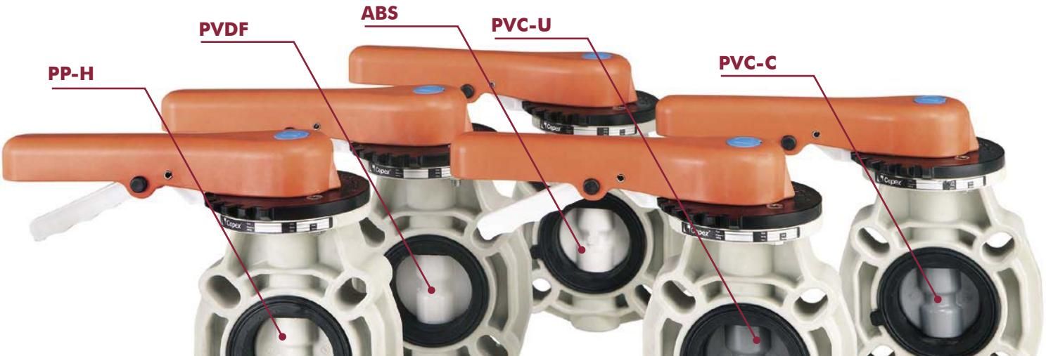
New range of butterfly valves in its Industrial Series (stainless steel shaft, food grade EPDM or Viton® sealing, PP - GF body & disc available in several materials). Sizes from D63 up to D315 (2" to 12"). The valve represents a major step forward both for its design and new features, offering the following characteristics:
